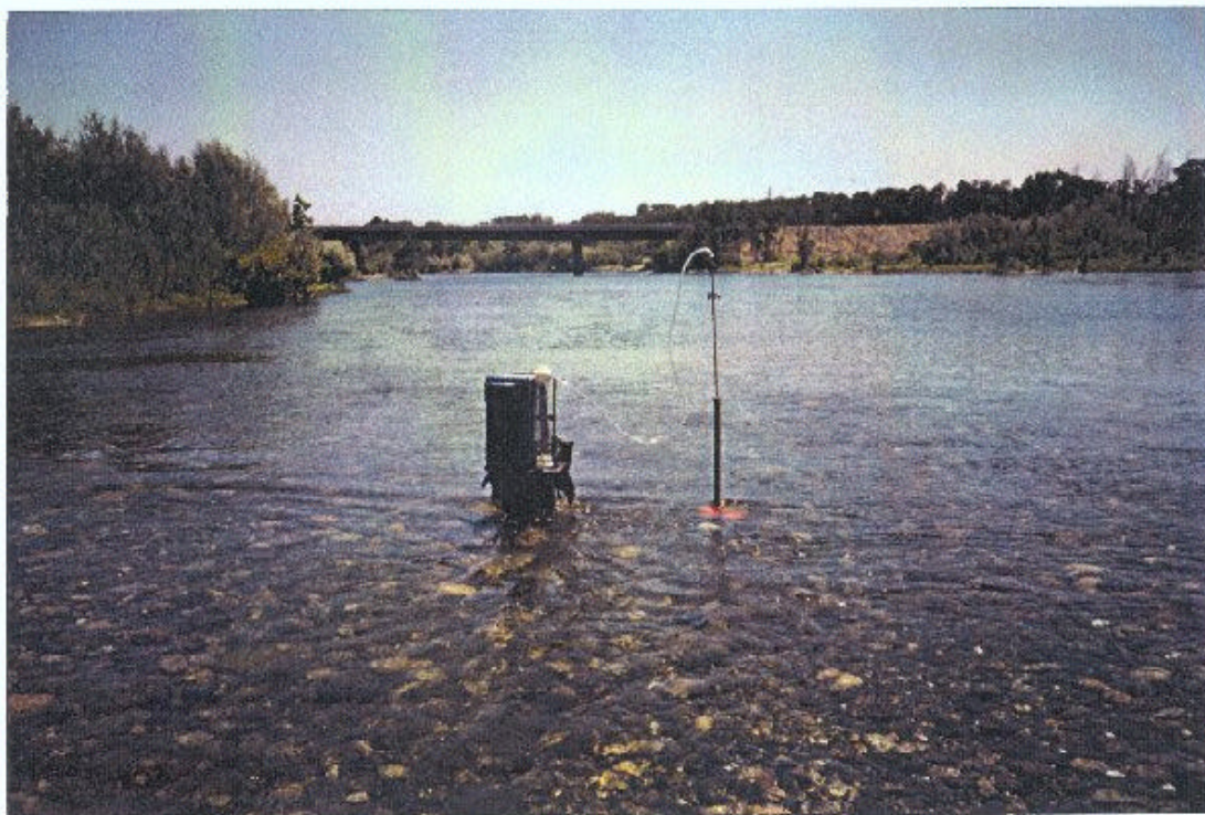
Photo 1. Modified Mark IV standpipe and electric pump assembly
