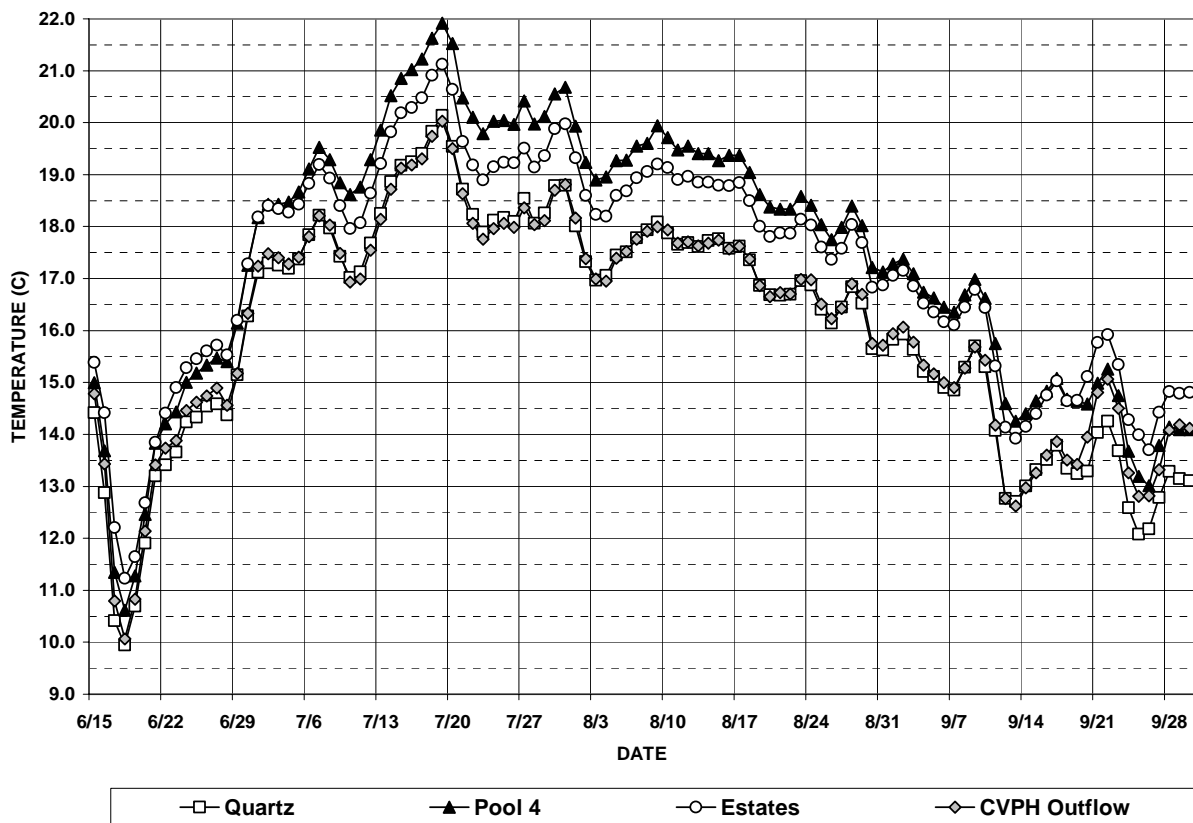
Figure 6. Mean daily water temperatures (C) at select SRCS holding pools in Butte Creek from June 15, through September 30, 2005.
